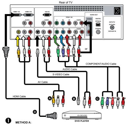
Use a composite cable to connect the DVD player's composite video/audio jacks to the LCD TV's VIDEO2 IN jacks.
